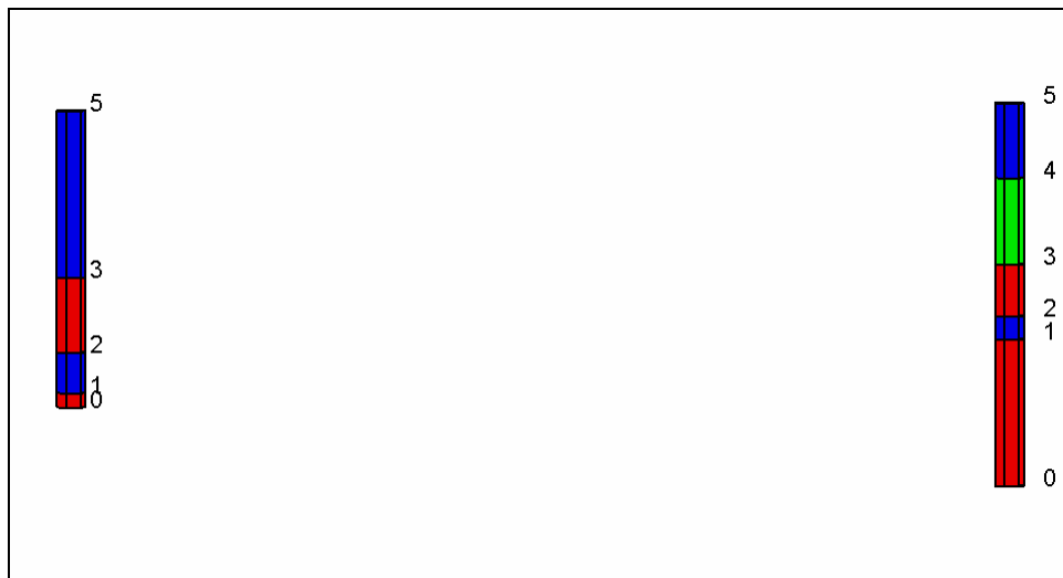
Figure 2. Two sample boreholes with horizon IDs assigned.
