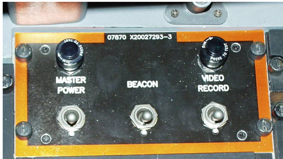
Figure B-6. Pacer Instrumentation Master Power Panel (Front Cockpit)
