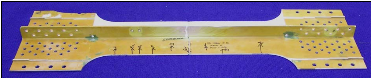
Figure 7. Revised Specimen Design with an 18-Inch Gage Length.
