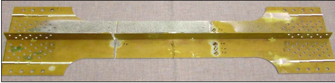
Figure 6. Example Specimen of 24-Inch Gage Length Design.
