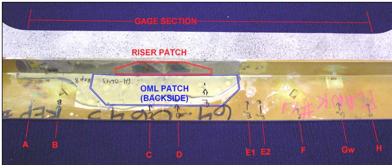
Figure 22. Typical Layout of Gage Length Cross Sections and Locations.
