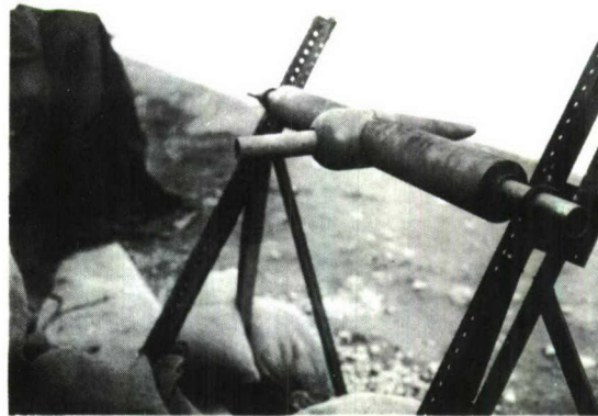
Figure 15 - X-band silicon carbide electromagnetic probe
