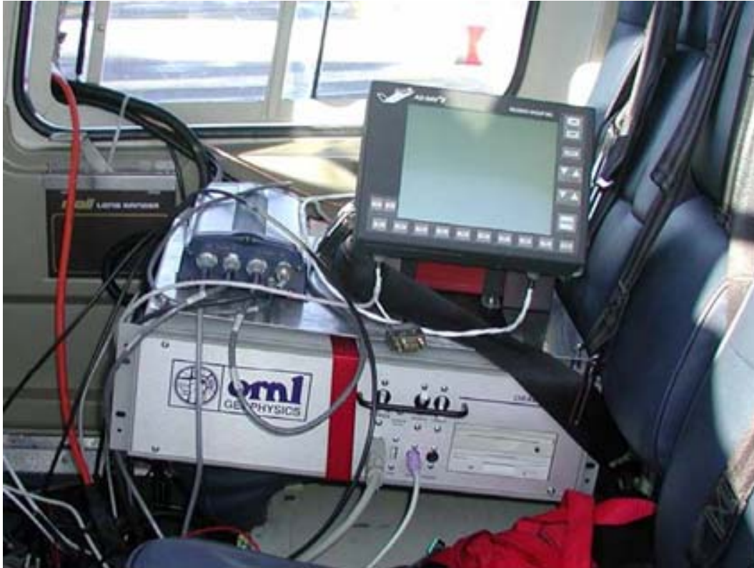
Figure 5. ORAGS-Arrowhead console as installed in the Bell 206 Long Ranger helicopter.
