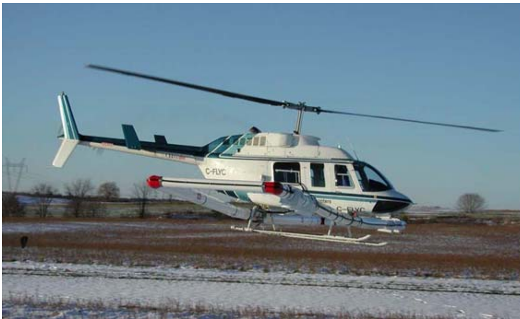
Figure 6. ORAGS-TEM airborne EM induction system similar to that used at Fort Ord.
