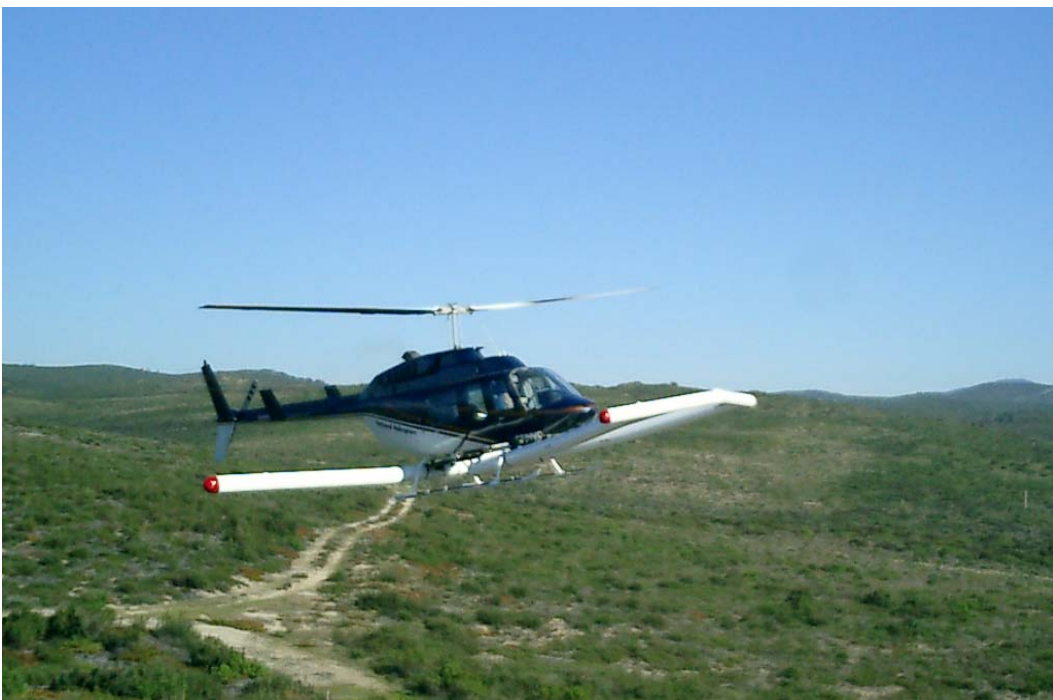
Figure 3. ORAGS-Arrowhead system in operation at Fort Ord.
