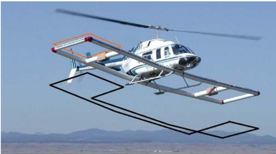
Figure 7. ORAGS-TEM system in flight. The red square shows the large receiver coil position, and the black line represents the rectangular two-lobed transmitter coil layout.
