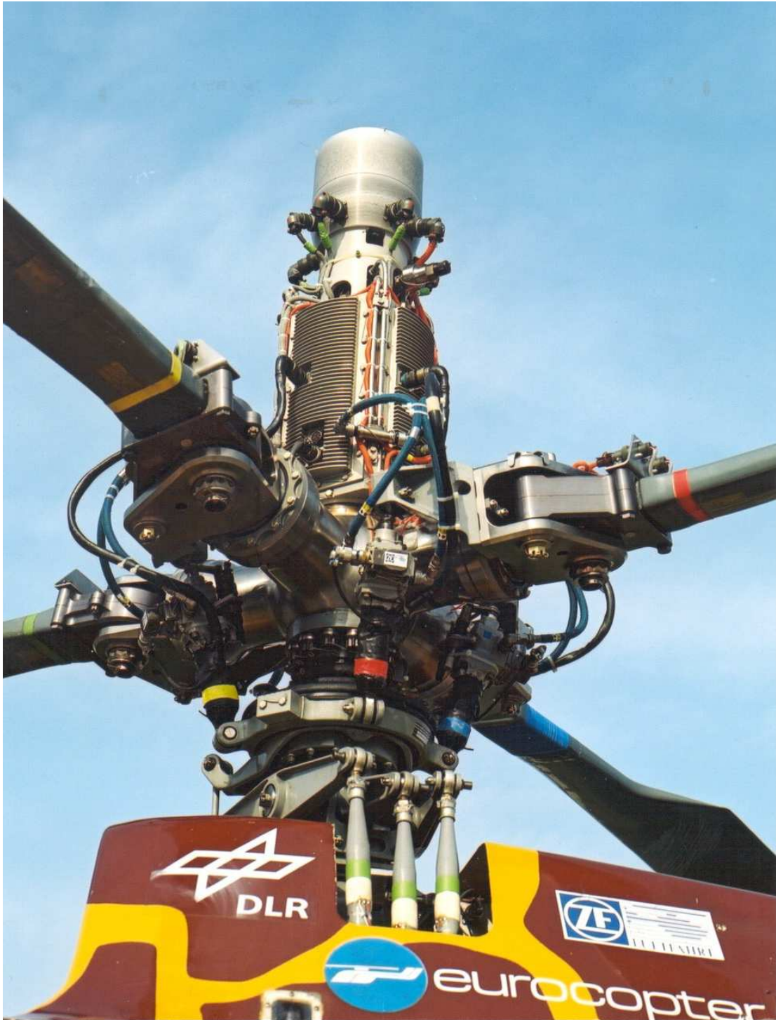
Figure 2.6: BO 105 Rotor Head With Dynamic Pitch Linkages [20].
