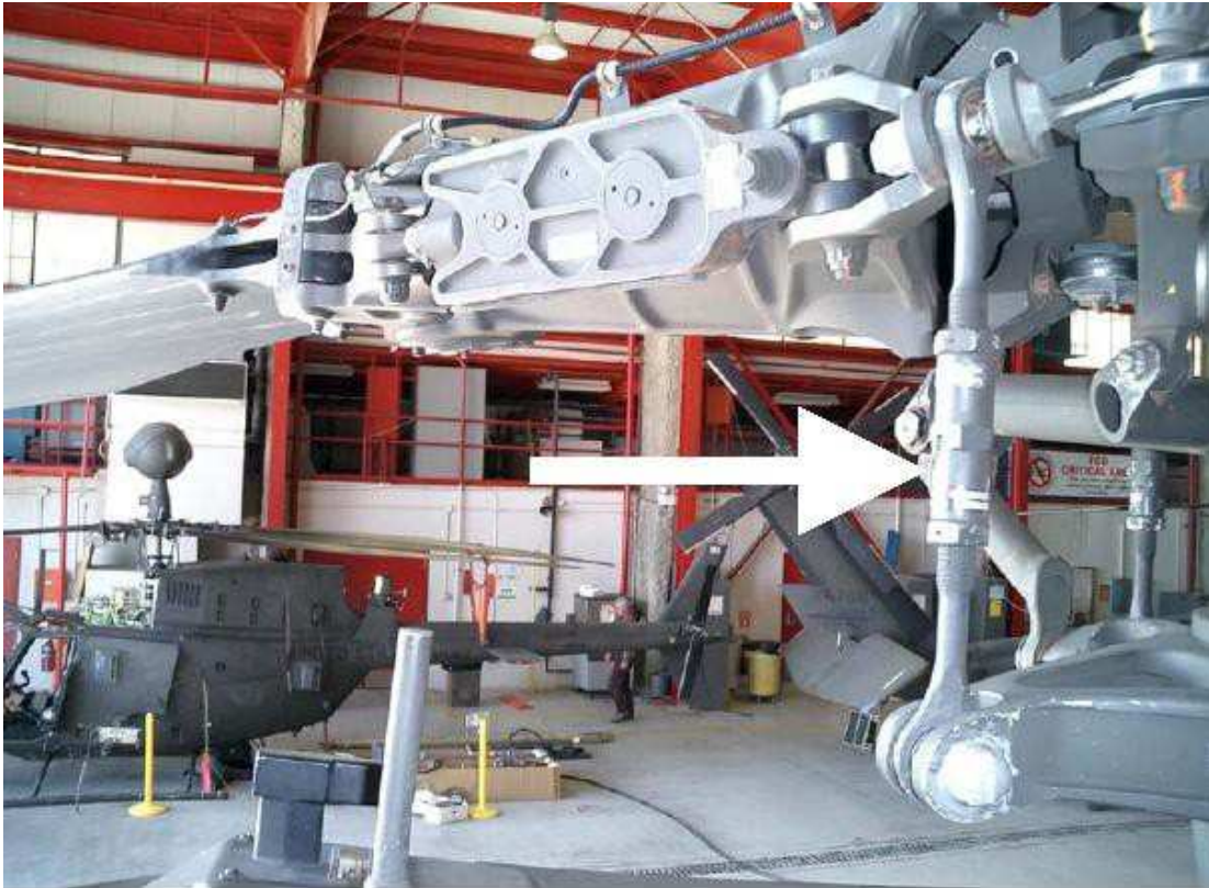
Figure 2.4: Rotorcraft Pitch Linkage Adjustment [23].
