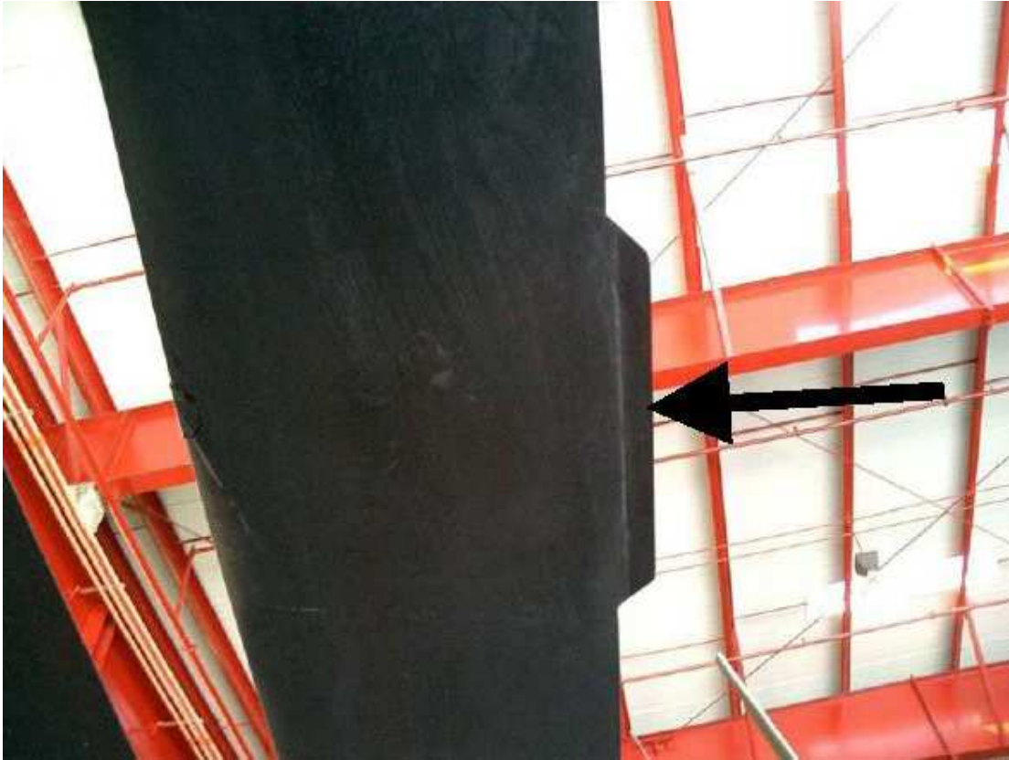
Figure 2.8: Rotor Blade Trim Tab at Trailing Edge [33].
