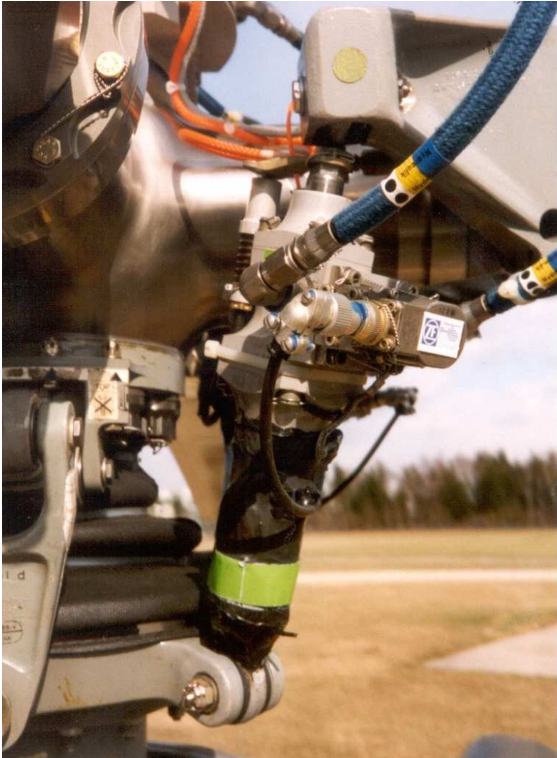
Figure 2.7: Individual Dynamic Pitch Linkage on a BO 105 [20].
