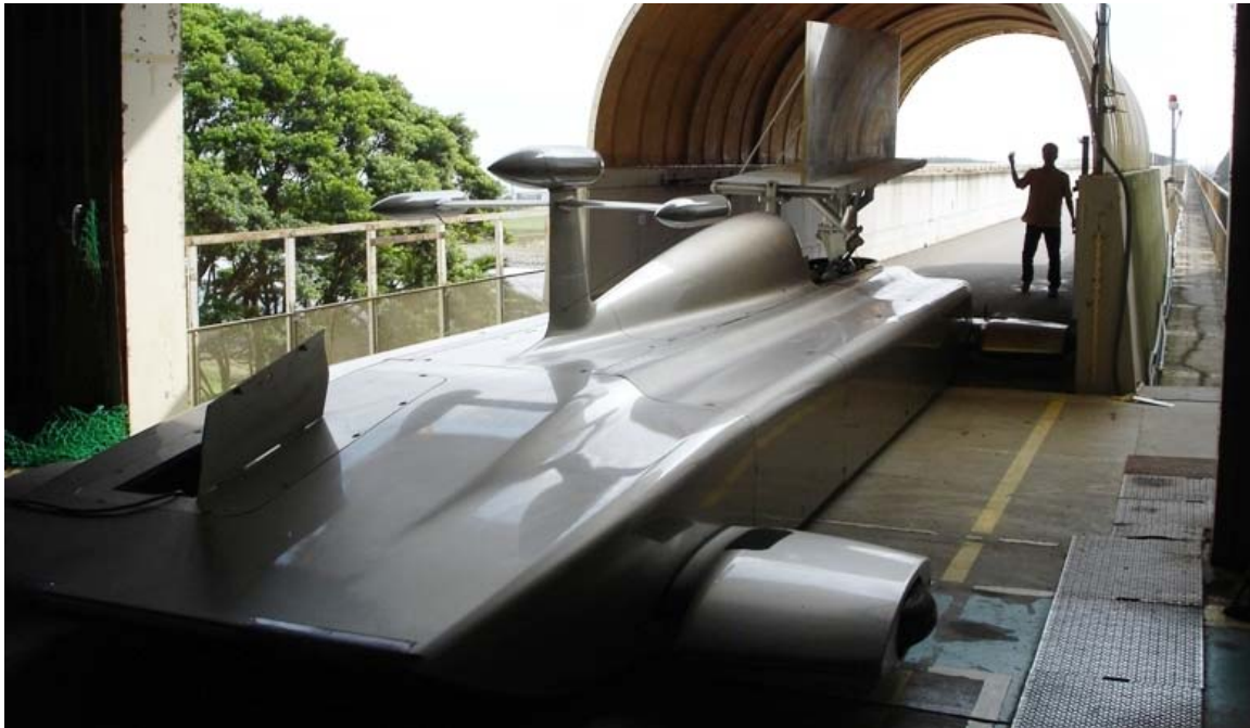
Figure 5. HART vehicle moving to beginning of test track with facility's flat plate model
