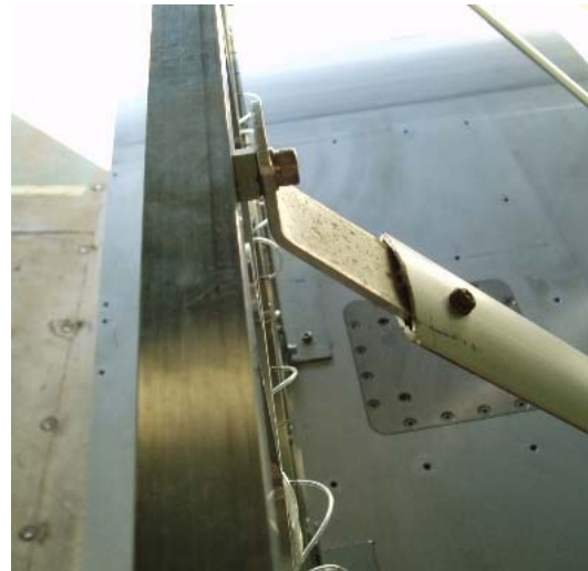
Figure 10. Washer used to set incidence
