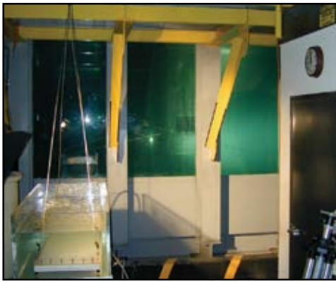
The Acoustic Division's Salt Water Tank Facility is designed for studying underwater acoustics in controlled, saline environments. Currently, this facility is being used to make measurements of sound propagation through bubble clouds.
