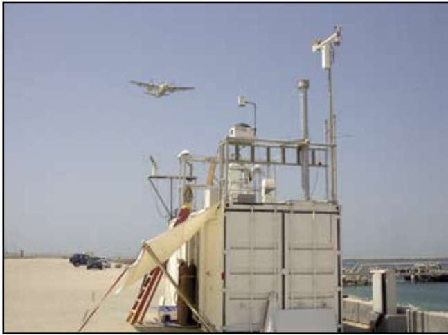
The Mobile Atmospheric Aerosol and Radiation Characterization Observatory (MAARCO) on deployment near Abu Dhabi, UAE, in August through October 2004, to gather data to support research on atmospheric aerosols, gases, and radiation. An instrumented Aerocommander is conducting an overflight.
