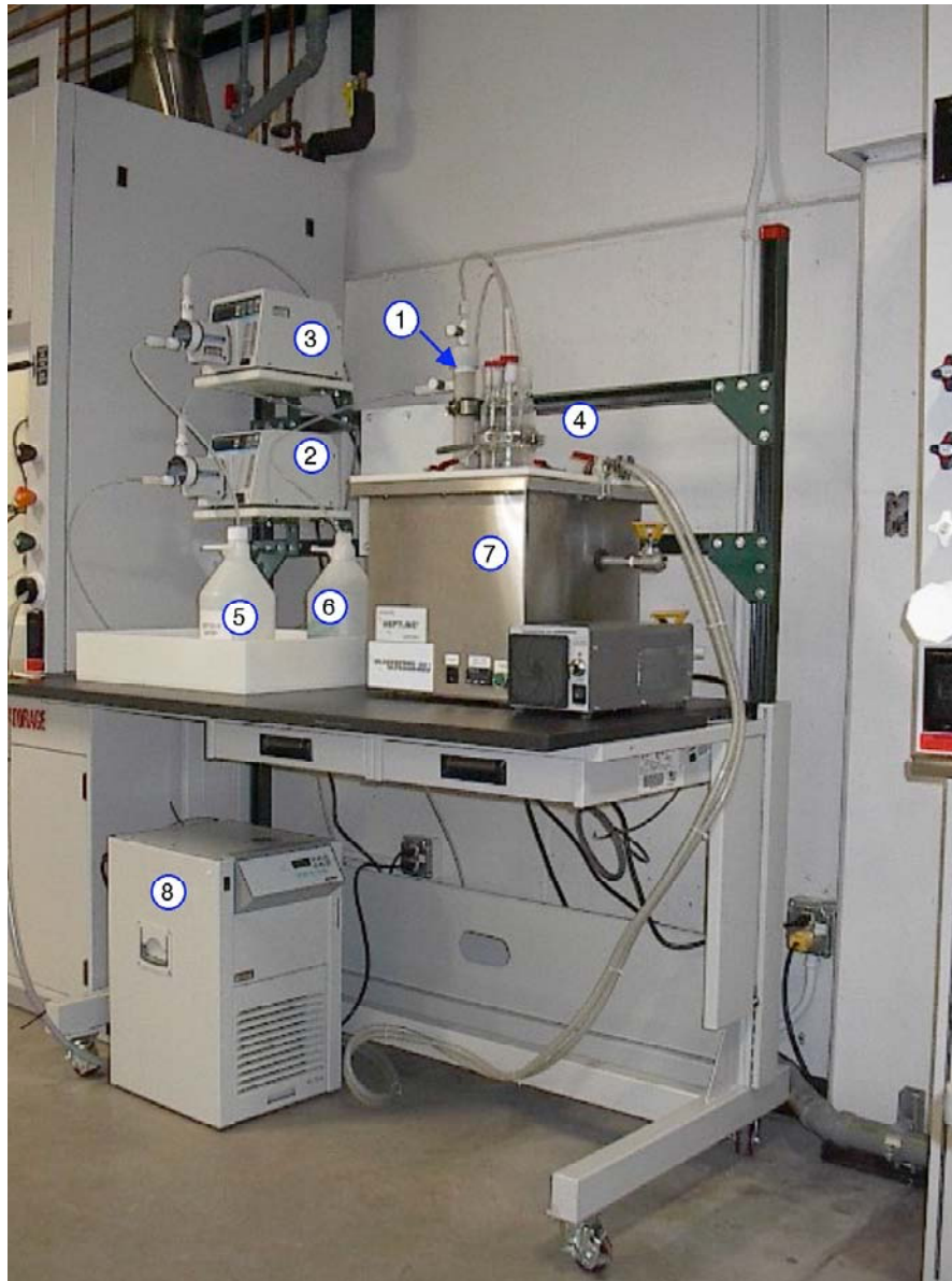
Figure 3. Original cross-flow filtration process equipment design
