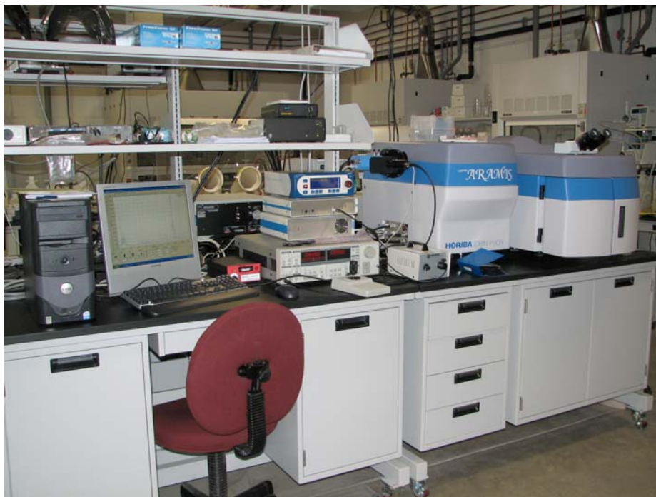
Figure 9. Raman spectroscopy measurement setup
