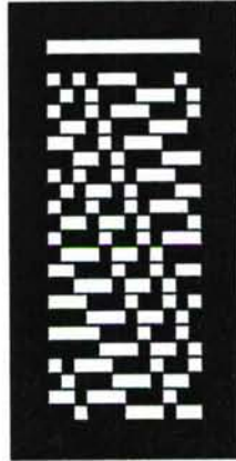
Figure 4.2: Diagram of a row-doubled Hadamard aperture mask based on an order-12 Hadamard matrix. White areas indicate light transmission, and black areas indicate where light is blocked.
