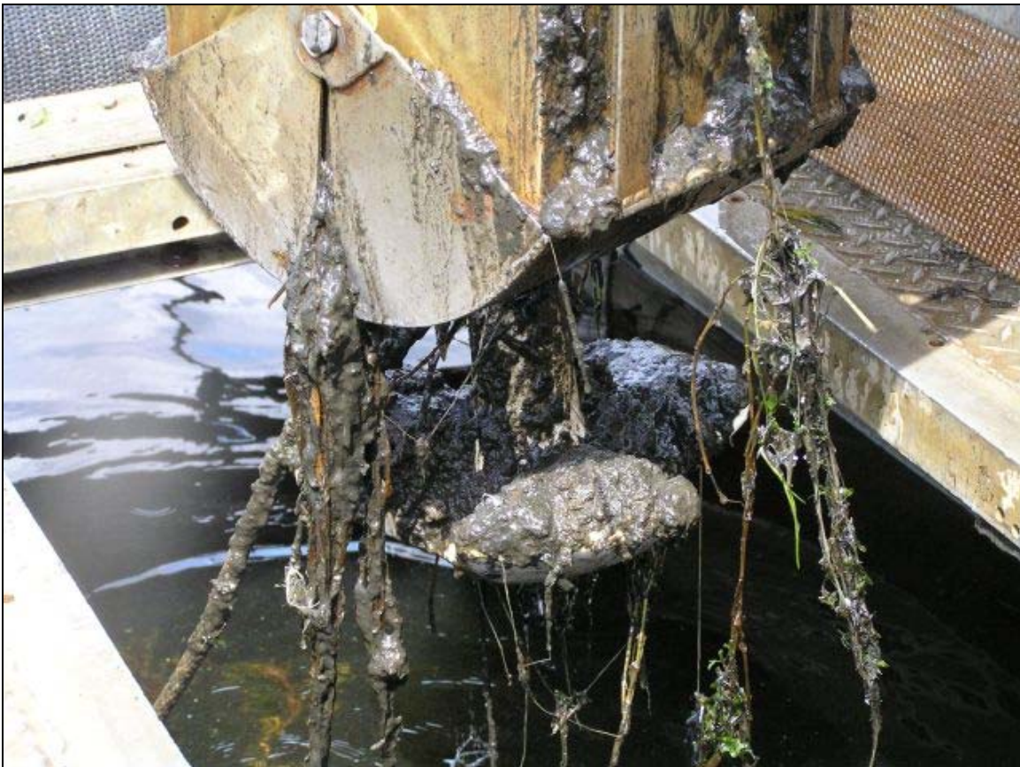
Figure 4. Box-core sampler after being deployed to capture plant sample.
