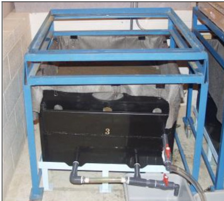
Figure 3. Lysimeter showing rainfall simulator holding frame and water collection system.
