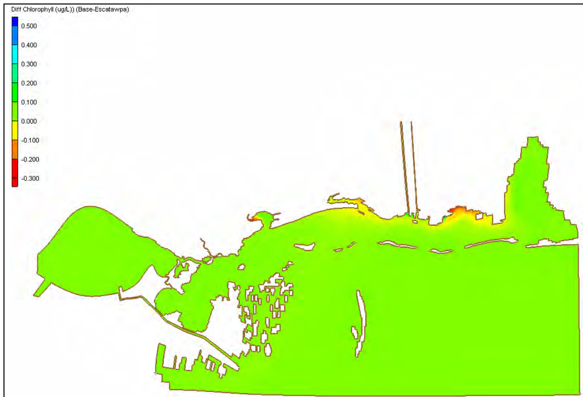
Figure 5-22. Difference in chlorophyll a ( \mu\text{g/L} ) from base condition resulting from Escatawpa River diversion (base minus diversion).
