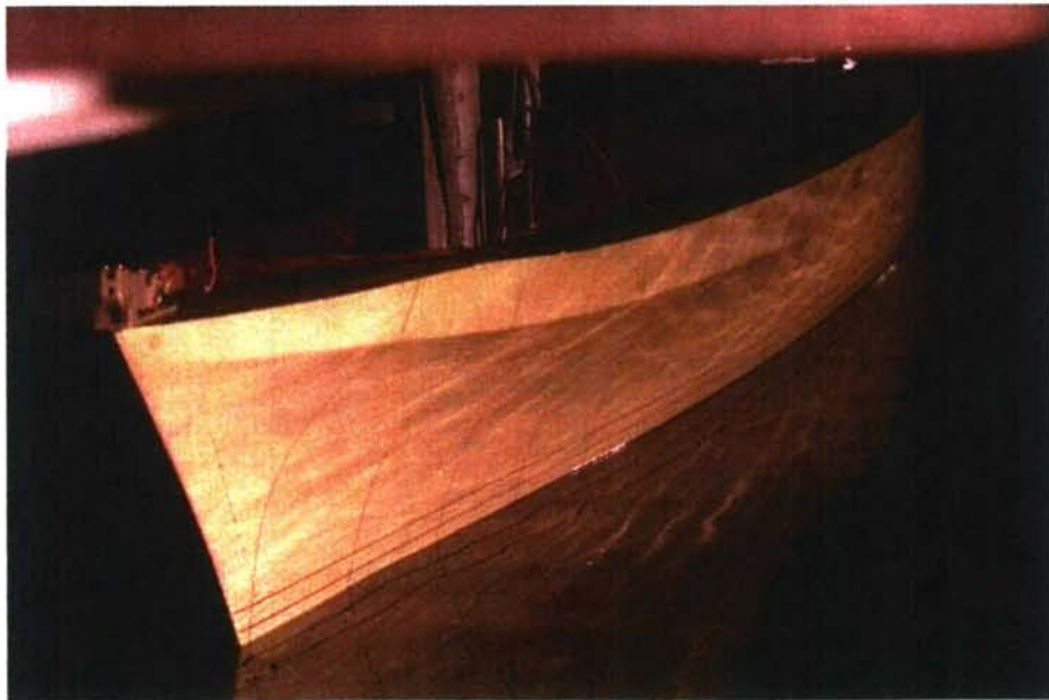
Figure B-2 - Bow wave at 2.09 knots (3.53 fps) model scale corresponding to 6 knots (10.1 fps) full scale; Vertical Displacement at FP= -0.059 in (-0.15 cm); Vertical Displacement at AP= -0.036 in (-0.09 cm)
