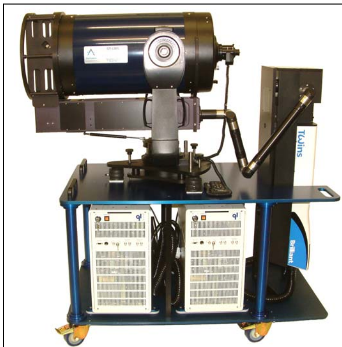
Figure 1. Photograph of the Gen 2 double pulse ST-LIBS system developed by ARL in collaboration with Applied Photonics, Ltd, and Ocean Optics, Inc.
