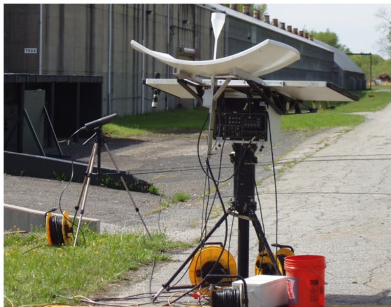
Figure 16. Dish antenna for telemetry data acquisition.
