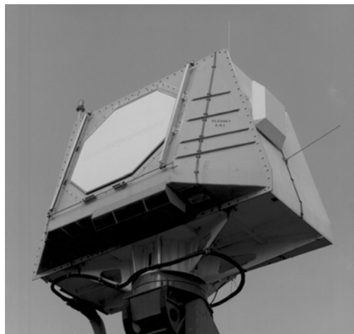
Figure 2: The MESAR (Multifunction Electronically Scanned Adaptive Radar) Active Phased Array Radar.
