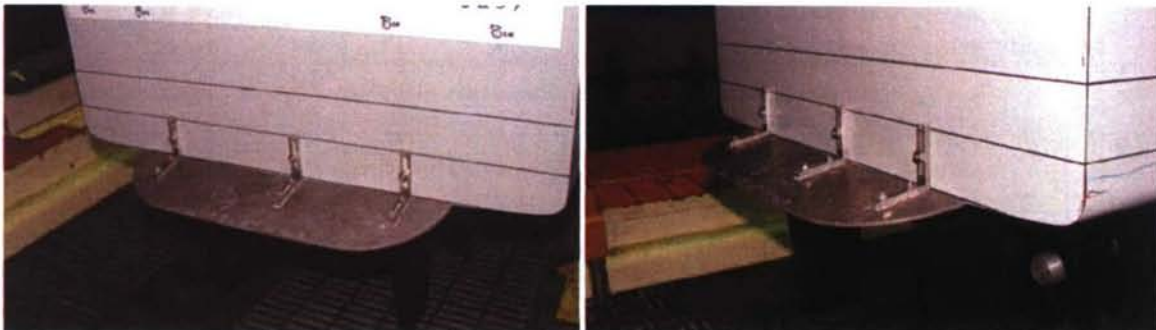
Fig. 4. Selected Stern Flap#4 at 10° trailing edge down
