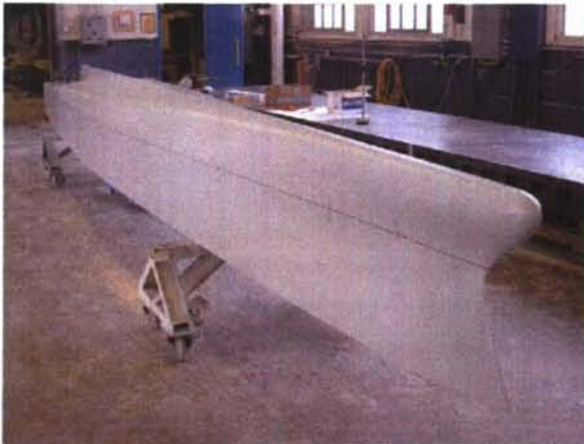
Fig 1. JHSS BSS Model 5653, bare hull shell
