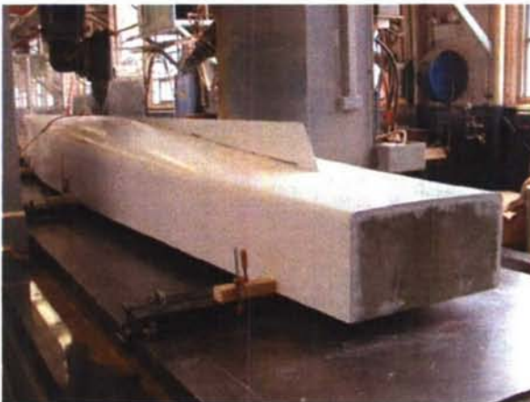
Model 5653 fiberglass shell removed from mold
