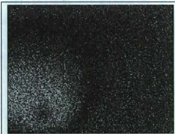
Figure 3-1: TOF-SIMS image formed by filtering on the mass of angiotensins. This rectangle is 200 microns on a side.
