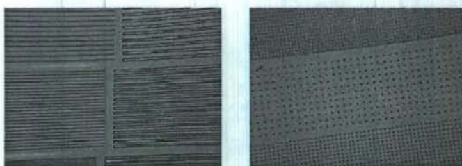
Figure 2-2. Microscopy photos of PDMS stamping of APES on SiO 2 surfaces. All features are less than 10 microns in size.
