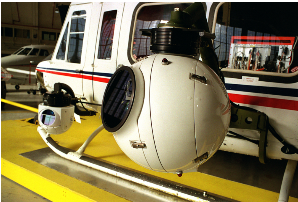
Figure 3. The 16- and 24- inch platforms that hold the thermal and AGTV imaging sensors respectively.
