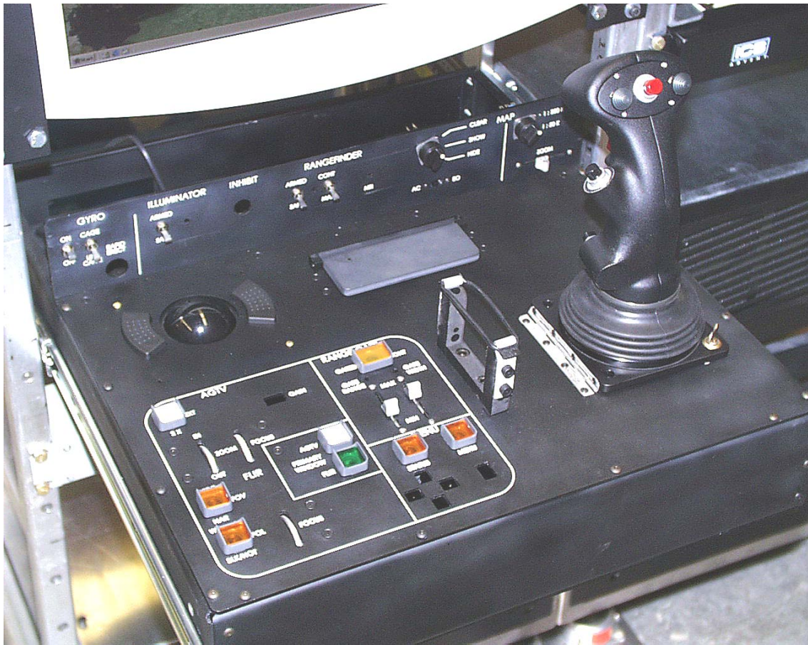
Figure 9. ELVISS console. This is the intended design. Prior to the trials, the sliders were replaced with rocker switches because of an incompatibility with the AGTV.
