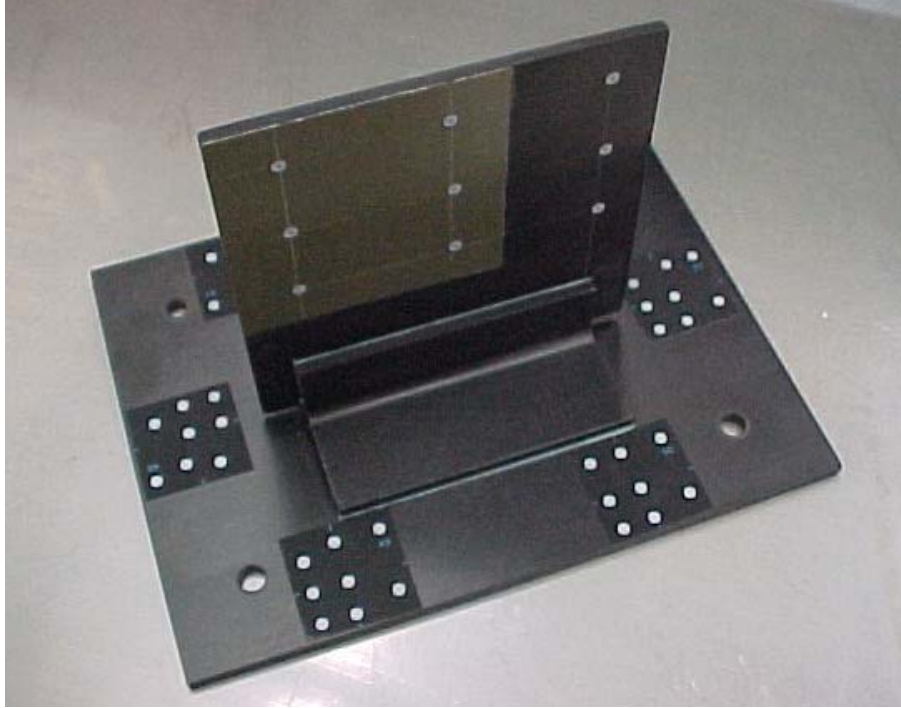
Figure 21. Composite T-joint prepared for thermal distortion testing
