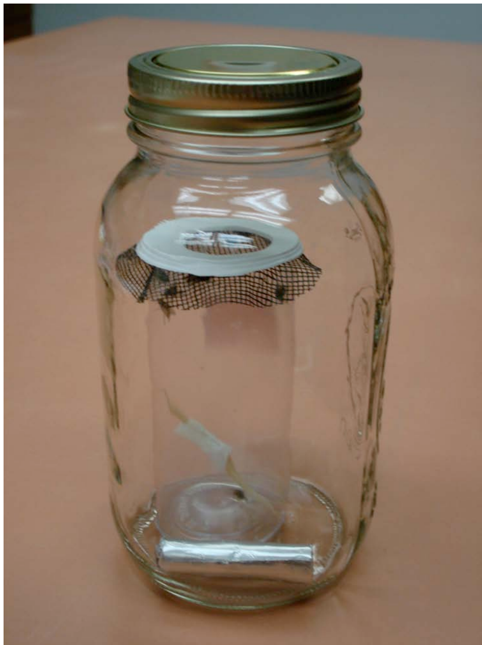
Figure 5. Mason jar set up to test controlled release of volatile for control of flies.
