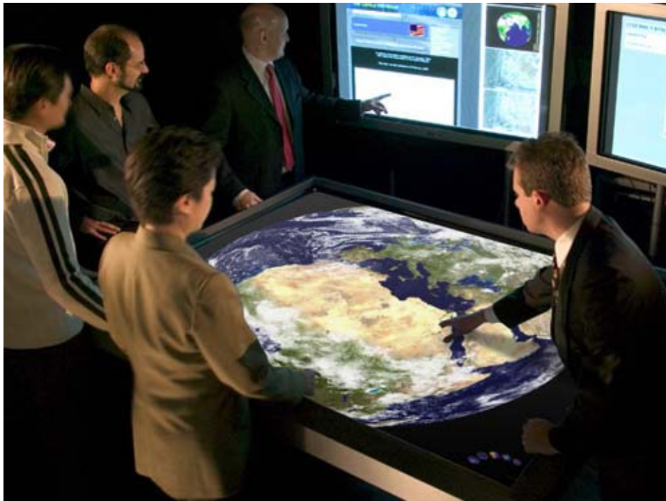
Figure 10. The Northrop Grunman TouchTable Users can draw, measure and interact with objects displayed on the touchtable. (source http://www.touchtable.com/ ).
