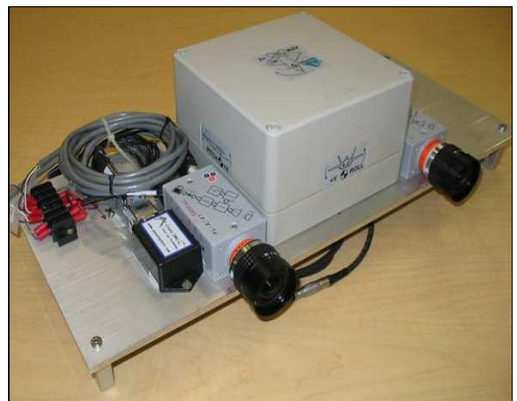
Figure 4: Data collection system. The data collection system consisted of a consumer-grade MEMS IMU and monochrome digital cameras. Although not used in this paper, a tactical-grade IMU was co-mounted on the platform in order to provide a performance comparison between different grades of inertial sensors.
