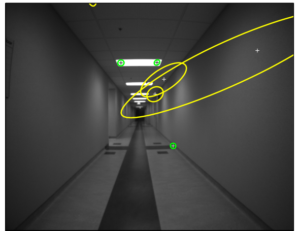
Figure 9: Sample image from indoor data collection. The indoor data collection presents the filter with man-made features in an office environment. The crosses and ellipses indicate the locations and uncertainty of currently tracked landmarks.
