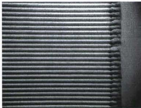
Figure 22. Stripes imprinted in a green YAG ceramic.
