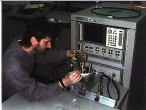
Fig. 21 High frequency test station with network analyzer (a) and split cavity probe fixture (b). The RF test station is used for dielectric characterization of substrate and thin film samples in the frequency range between 1 GHz and 38 GHz.
