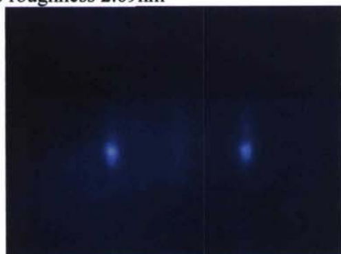
(b) “Streaky” (11-20) RHEED indicates low growth surface roughness, 2D step flow growth mode
