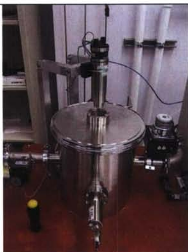
(c) (d) Fig. 04 Hydrogen etching system (a – schematic, b – typical process sequence, c – vacuum chamber, d – etcher assembly) for the ex-situ preparation of clean, atomically flat substrate surfaces for MBE growth experiments.
