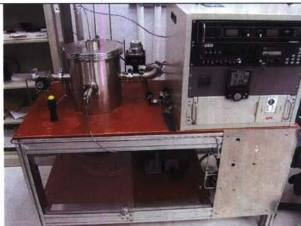
(c) (d) Fig. 04 Hydrogen etching system (a – schematic, b – typical process sequence, c – vacuum chamber, d – etcher assembly) for the ex-situ preparation of clean, atomically flat substrate surfaces for MBE growth experiments.
