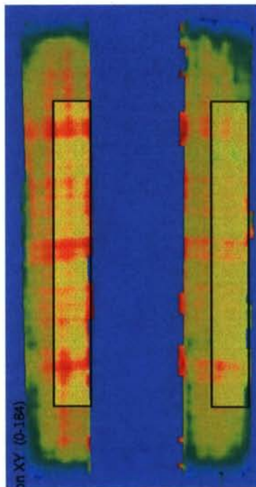
Figure 2.6: Full-Field Shear Strain of a D4255 Specimen
