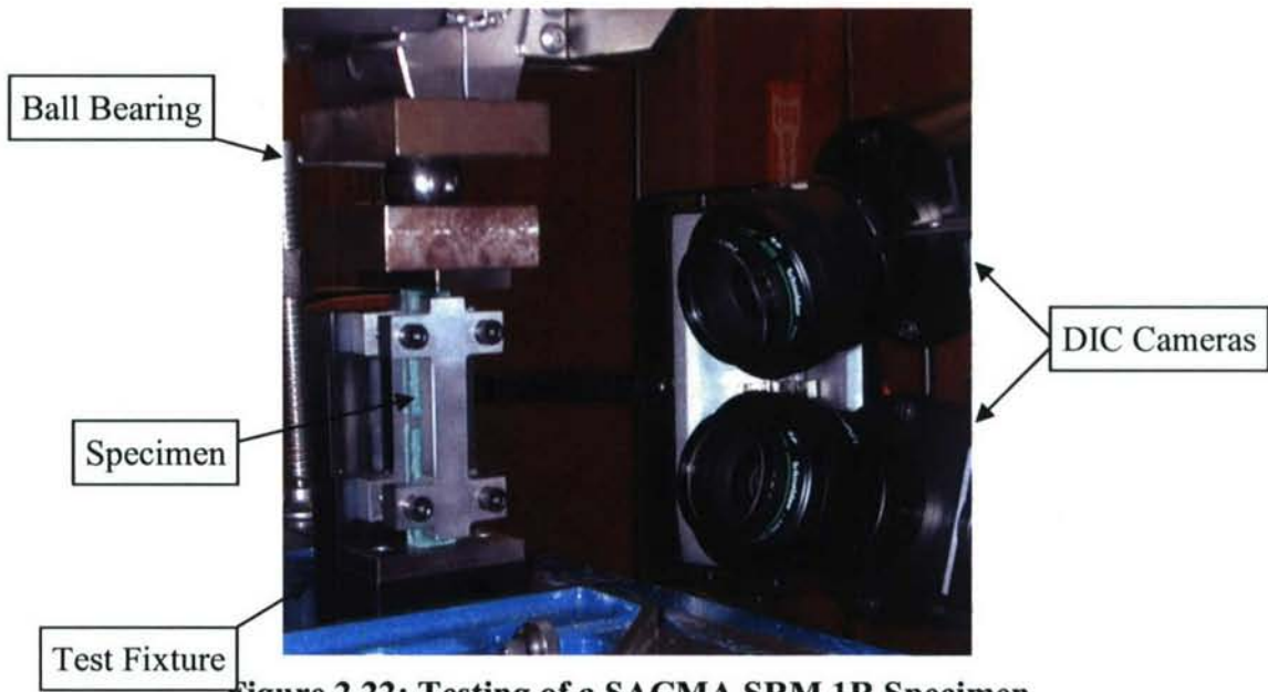
Figure 2.22: Testing of a SACMA SRM 1R Specimen
