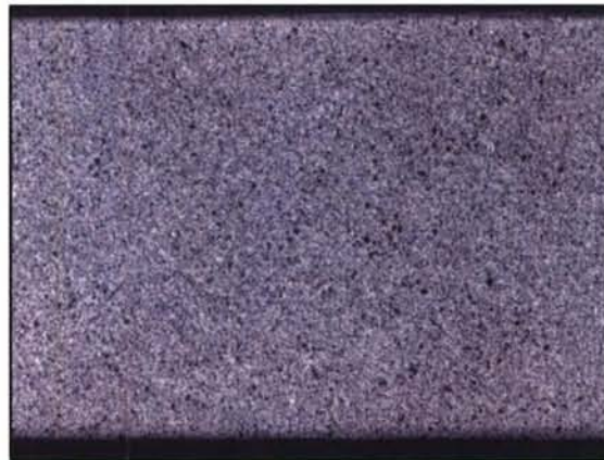
Figure 2.51 Speckled Grayscale Pattern on Face of Specimen
