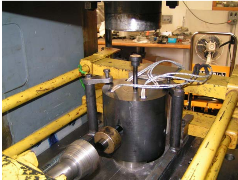
Fig. 9 Unit for elevated-temperature ECAE with back-pressure at Monash University
