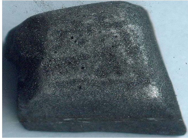
Fig. 13. Loss of shape and weight (54 w%) of a square shaped dense expose up to 1473K for 140 minutes.
