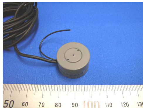
Fig.9 Micro CCD camera implemented on small robot to get the visual image around it
