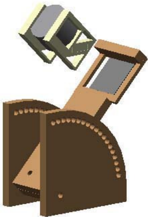
Fig.10 Isometric view of the leaf spring assisted catapult launching mechanism
