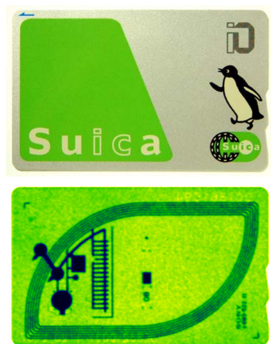
Figure 2. THz image of a Japanese railway payment card. The THz waves penetrate the plastic card and reveal the circuitry inside, including a 6-loop antenna for the touch-and-go feature of this card.
