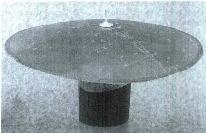
Figure 27. Prototype Membrane on Temporary Mount for Stowing
