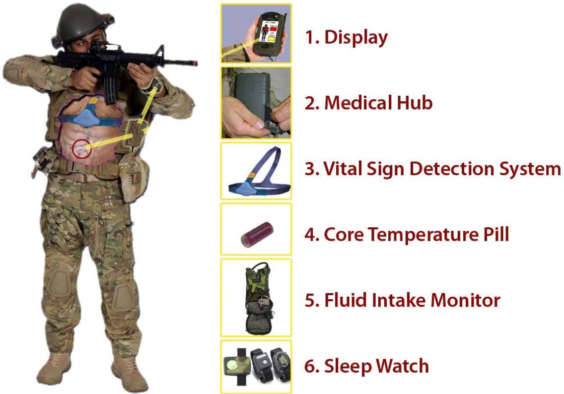
Figure 1. Warfighter Physiological Status Monitoring – Initial Capability system
