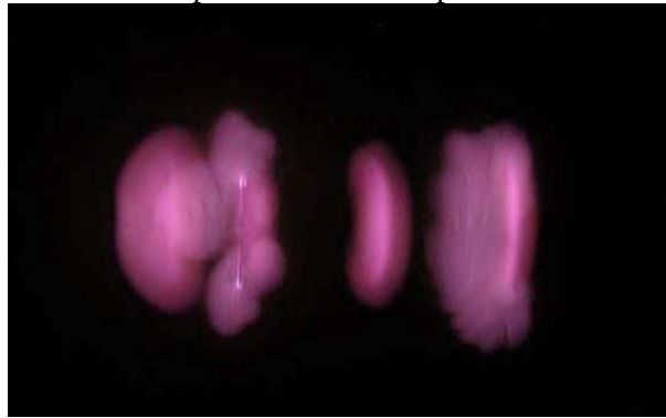
Fig.7.2.3.1. EM field structure visualizing in the working area at application of the diffuse discharge
