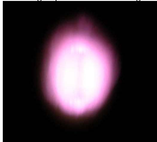
Fig.7.2.4.2. Appearance of longitudinal MW discharge from a bunch of EM pulses in a high-speed flow
