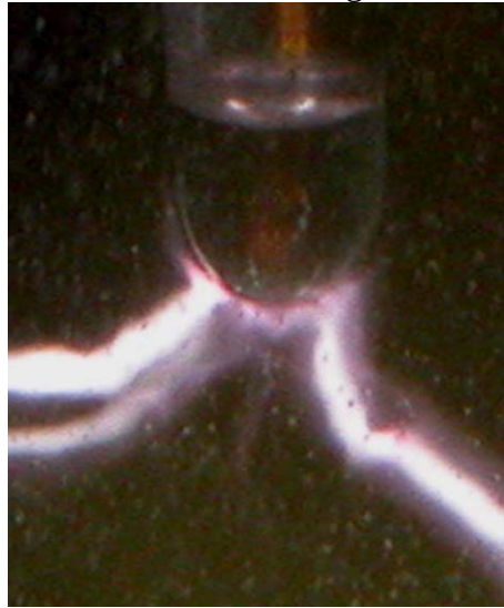
Fig.4.7.3. Undercritical discharge fragment near vibrator's surface at water drop in developed state on it
