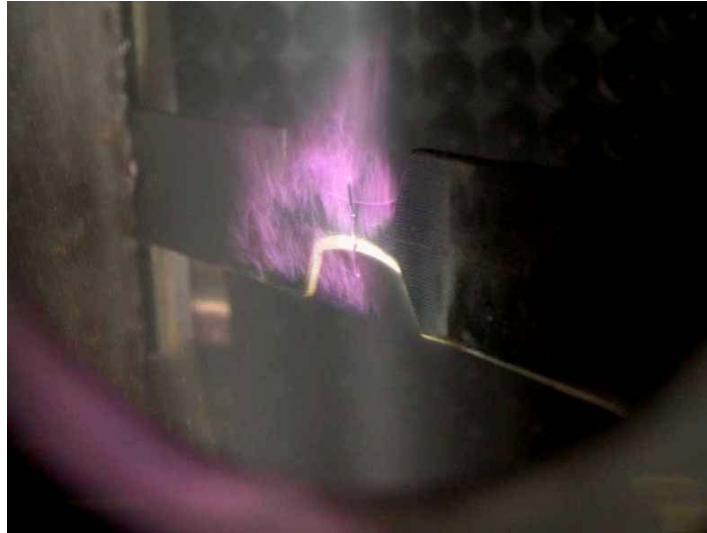
Fig.5.9.5.5. Appearance of the undercritical MW discharge in the high-speed air flow with v_{fl} \approx 500 m/s at presence of water aerosol in it
