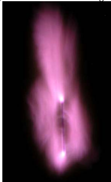
Fig.7.2.4.4. Appearance of longitudinal MW discharge from a bunch of pulses in a high-speed flow
