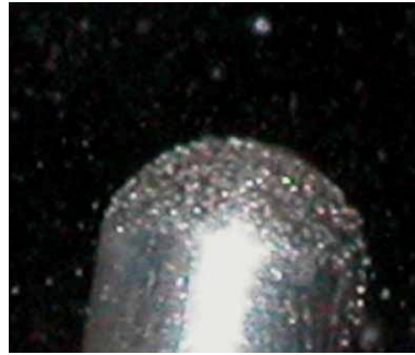
Fig.4.6.1. Appearance of the initiating vibrator surface covered by separate water aerosol particles deposited on it
