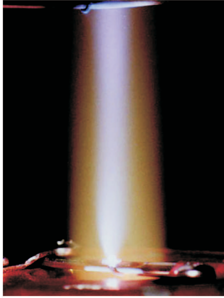
Figure 2.13: DC glow discharge in air (1.4 kV/cm, 200 mA). Interelectrode distance is 3.5 cm 79 .
