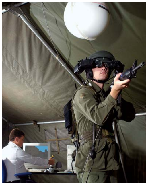
Figure 1: The Dismounted Soldier Simulator with Helmet Mounted Display, Weapon, Position Tracking Sensors, and Control Computer.
