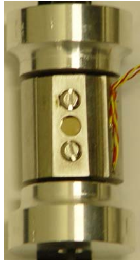
Figure 25: Hollowed cylinder and faceplate assembly
