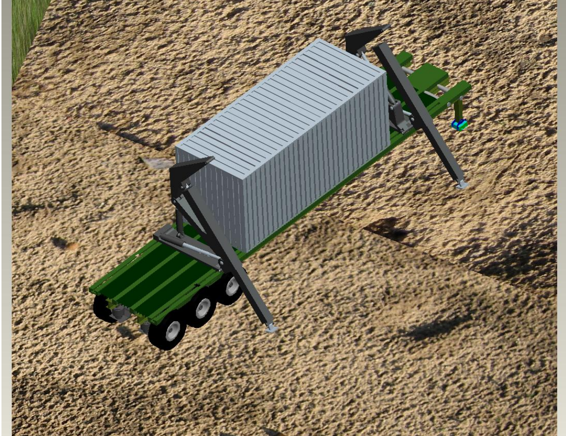
MFT Cranes after Loading 20 foot ISO Container
