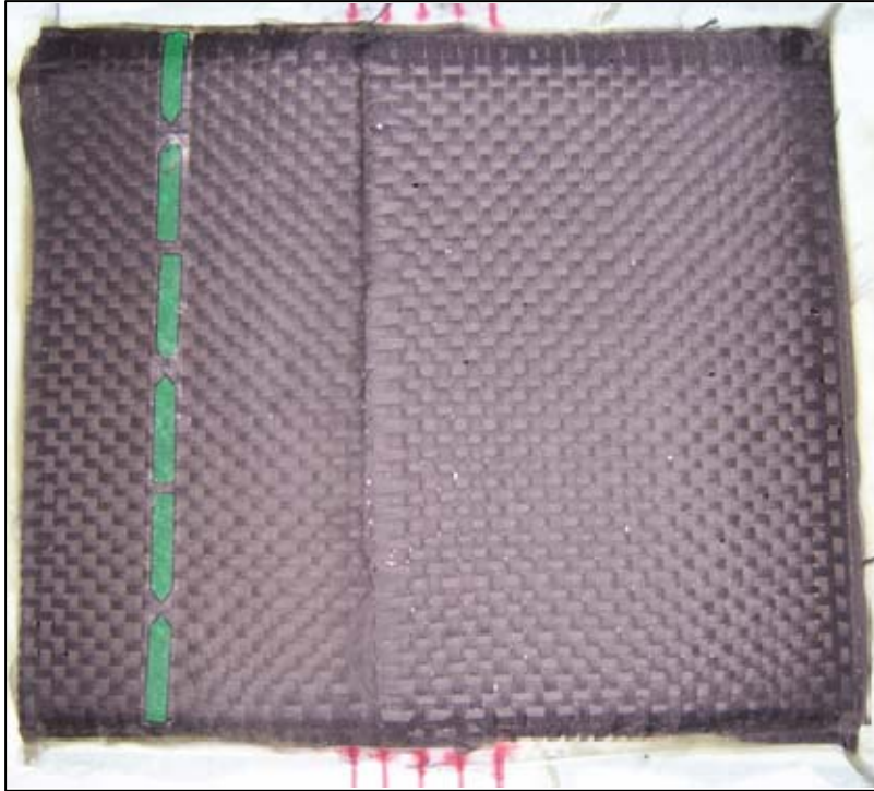
Figure 7. Complete Sheet (Following Vacuum Curing)
