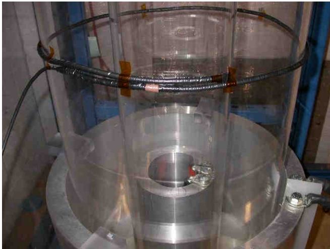
Figure 3. Photo of the inner and outer discharge coils mounted with the annular quartz vacuum chamber. Also shown is a 40 cm Rogowski-coil and high-frequency electro-magnetic shielding
