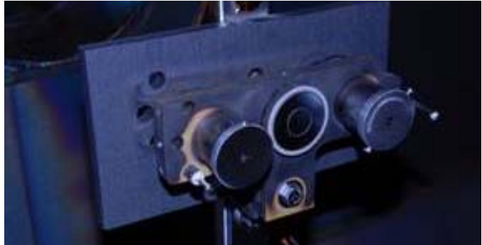
Figure 2. Plasma diagnostic array at AFRL. Probes from left to right include: Langmuir probe, RPA, nude Faraday probe, and gridded Faraday probe.
