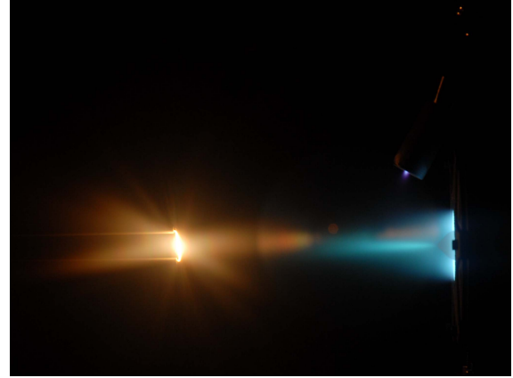
(b) Emissive probe heated during a hot I - V characteristic measurement.
