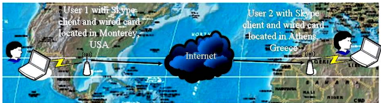
Figure 35. VoIP Measurements on a WAN Implementation. The Two Users are Located in Monterey, California and Athens, Greece, Respectively. One User Transmits a Recorded Message through VoIP Using Skype and the Other Records it.
