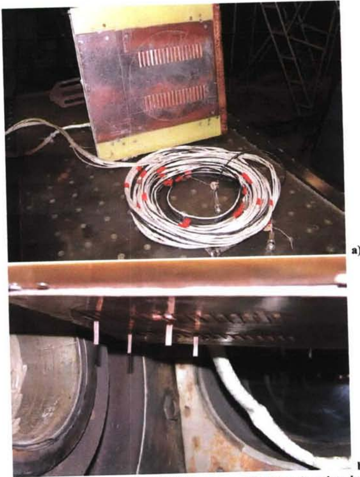
Figure 152. Model used at HFP WT after modification. a) equipped with flush mounted electrodes only; b) with additional pin electrodes installed at the 1st and the 10th electrode pairs in the test section
