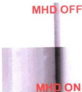
Fig.34. Imaging of the flow around cylinder with and without MHD interaction as recorded with Pulnix digital camera. The flow direction is from the right to the left.
