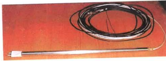
Fig. 104. Double probe for electron density and electron temperature measurements.
