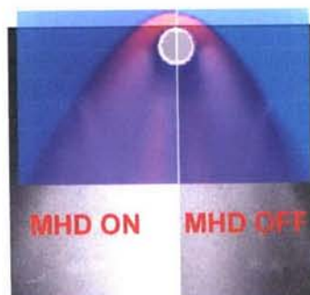
Fig.38. The visualization (b&w) and computation (colored) comparison of the wake area flow field under MHD-off and MHD-on conditions.
