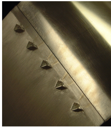
(b) Counter-Rotating VGs, 150% BL height, with Base Block
