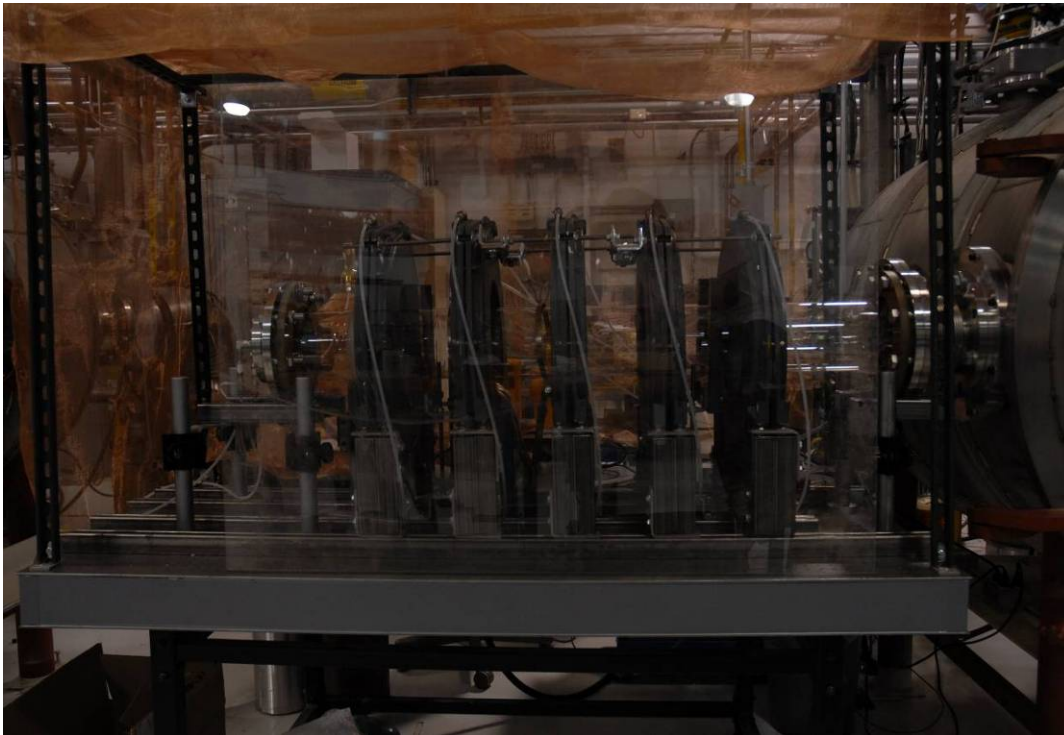
Figure 1. A 15-cm diameter helicon source.
