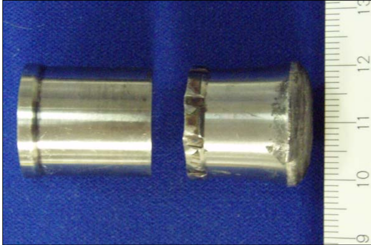
Figure 9a. Photo of a real initial FSP (left) and real residual FSP (right).
