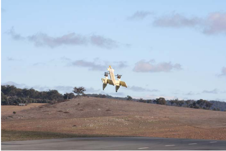
Figure 4: T-Wing landing while tilting into wind
