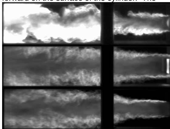
Figure 6-2, High Speed Images of the Circular Cylinder, Square Cylinder and V-Gutter at Re = 30,000 , Equivalence Ratio = 1.0
