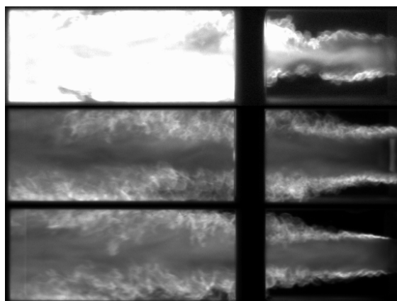
Figure 6-1, High Speed Images of the Circular Cylinder, Square Cylinder and V-Gutter at Re = 20,000 , Equivalence Ratio = 1.0
